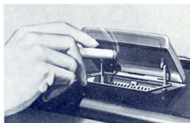
FAST-ACTING CIGARETTE LIGHTER (note control console)
